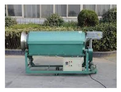
• **Tea Roller-** The Rolling Machine is used to crank up leaves rolled into a bar and broken cells, with controlled process parameters such as the cable tight knot, low broken tea, and so on. It is suitable to all types of rolled tea processing, and the rub ribs level must be specified during the purchase.
